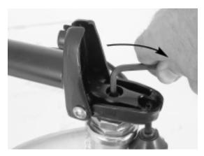
Figure 3. Tighten the wedge using a 6mm allen wrench.
